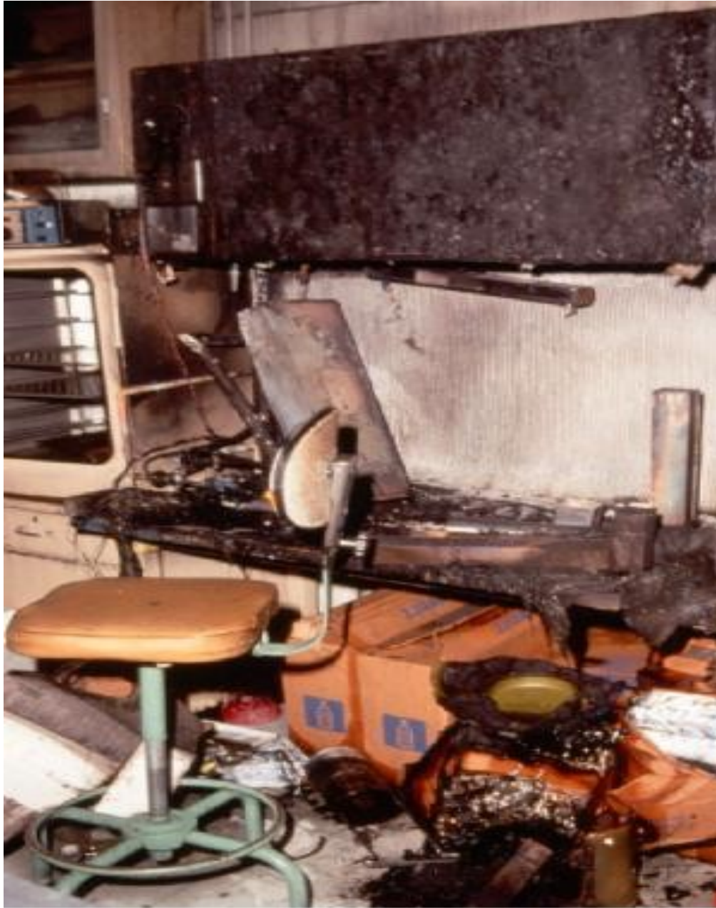
Fire in a Biosafety Cabinet
